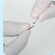
Open-end Kapillare abbrechen
