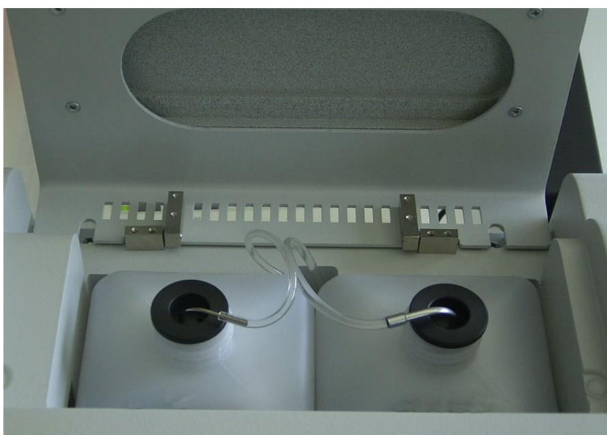
Fig. 6.3 View of supply and waste container
